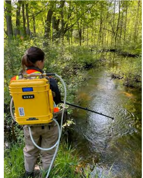
CH technician using an eDNA sampler to collect water samples in Bronte Creek
